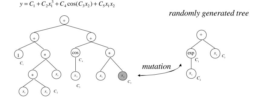
After: Mutant  $y = C_1 + C_2 x_1^3 + C_3 \cos(C_4 x_2) + C_5 x_1 \exp(C_6 x_1) + C_7 x_1^2$
